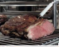
Multipoint cooking probe (Lev. 3), singlepoint (supplied as standard in Lev. 2, optional in Lev. 1) and vacuum (optional) = controlling product core temperature in all conditions.
